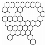
Fig.4 Structure of activated carbon [19]
