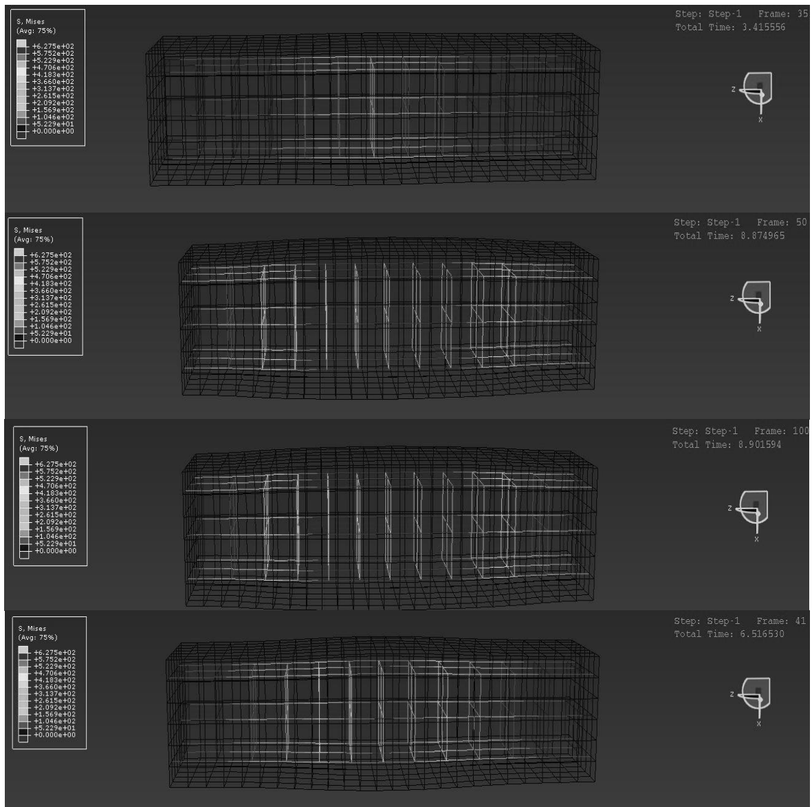
Figure 8 Behaviour of GFRP Rebars in Compression and Failure by Buckling at Different Load Stages
