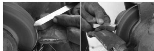
Figure 4 HSS tool shaped on grinding machine. [8]
