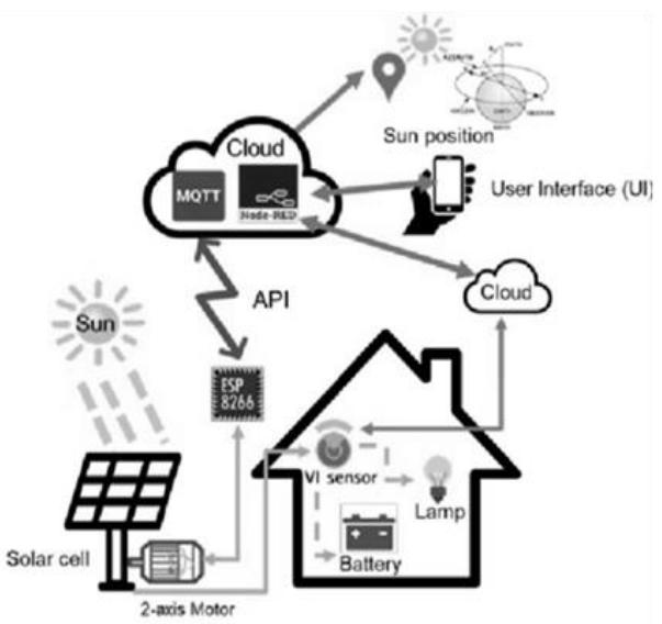
Our system constantly monitors the solar panel and transmits the power output to the IoT system over the internet. Here we use IOT to transmit solar power parameters over the internet to IoT. It now displays these parameters to the user using an effective GUI and alerts them when the output falls below specific limits. This makes remotely monitoring solar plants very easy and ensure the best power output.
