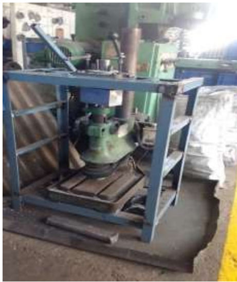
Fig.10 Experimental Setup of Special Purpose Spot Facing Machine
