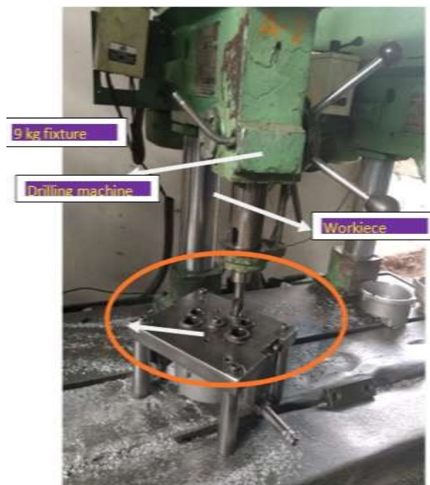
Fig.1 Existing Spot Facing Machine.
