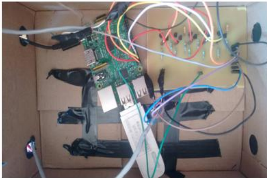
Fig. 4 '3G' dongle connected to raspberry pi
