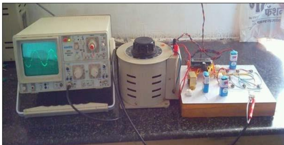
Fig. 10 Complete assembly of the experimental setup of 7-level inverter with output waveform
