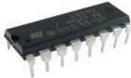
Fig.6. L293D motor driver
