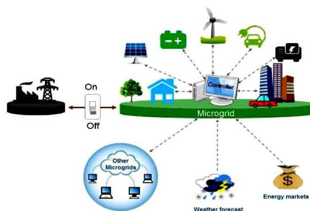
Figure 1: Schematic diagram of a DC microgrid system
