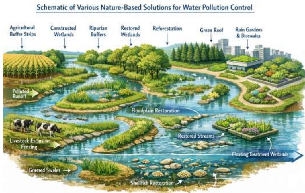
Figure 1: Schematic of Various Nature-Based Solutions for Water Pollution Control
