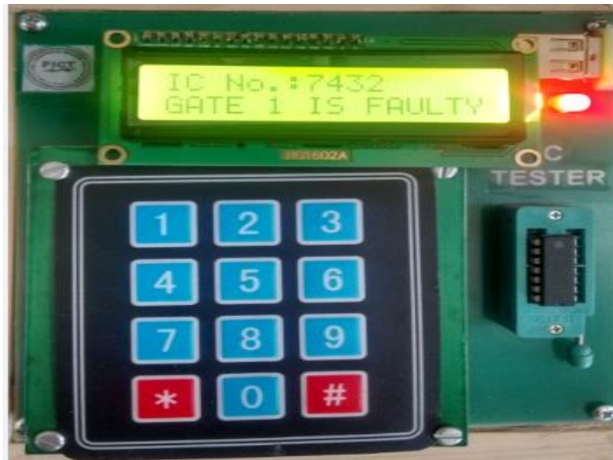
Figure 8: Testing of 7432 (Not-working IC)
