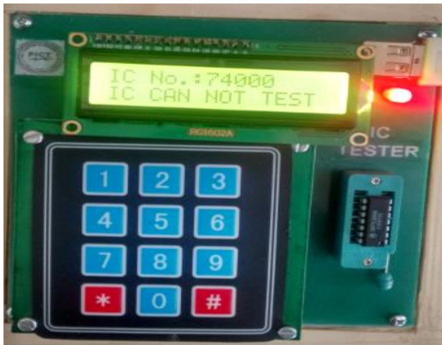
Figure 9: Result for incorrect IC number
