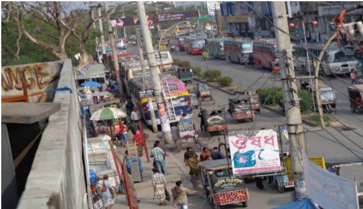
Fig. 13: Illegal Parking Reduces Capacity of Road at Station Parking Point.
