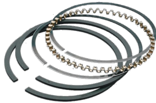
Figure 3. Piston ring examples [9]
