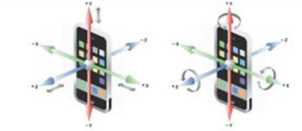
Figure no.3: Cartesian Coordinate Axes of Phone Accelerometer and Gyroscope
