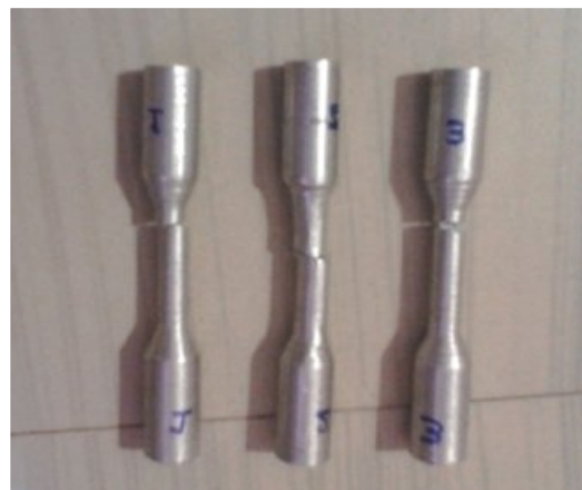
Fig-3 Broken composite specimens
