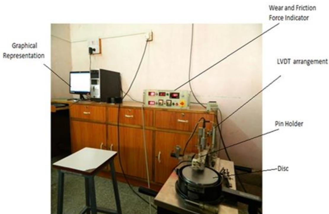
Fig. 1 Apparatus of pin on disc tribometer.
