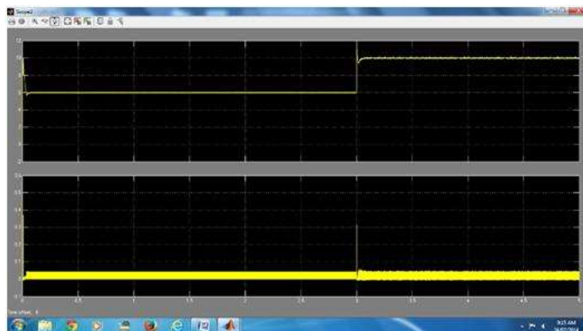
Figure 8 Output of DC-DC (buck) Converter using Proposed NNC
