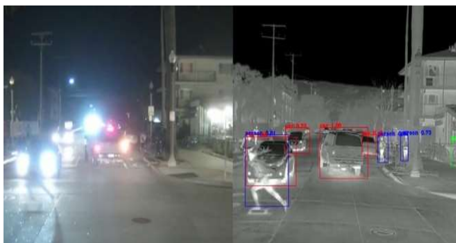
Fig.5 : View of Roads at night (a) General View, (b) Thermal View
