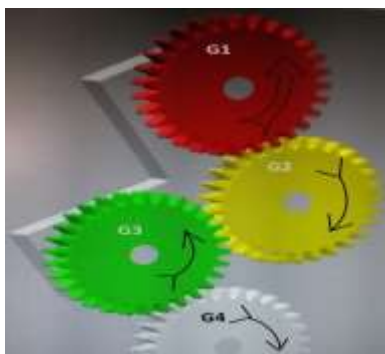
Fig.4.1.1:-Design of Reverse Gear for Trike in Design Software
