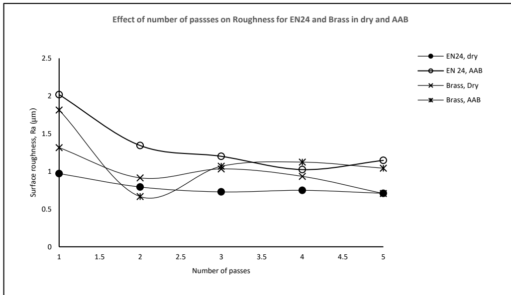
Figure 6: Effect of number of passes on Roughness for EN24 and Brass in dry and AAB (conditions constant Force;8 kgf, feed 0.119 mm/rev and speed 585 rpm)
