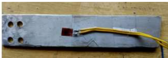
Fig.17. Load cell connected with cables
