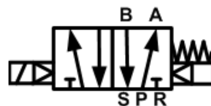
Fig 4.13 5x2 Solenoid operated spring return type DCV
