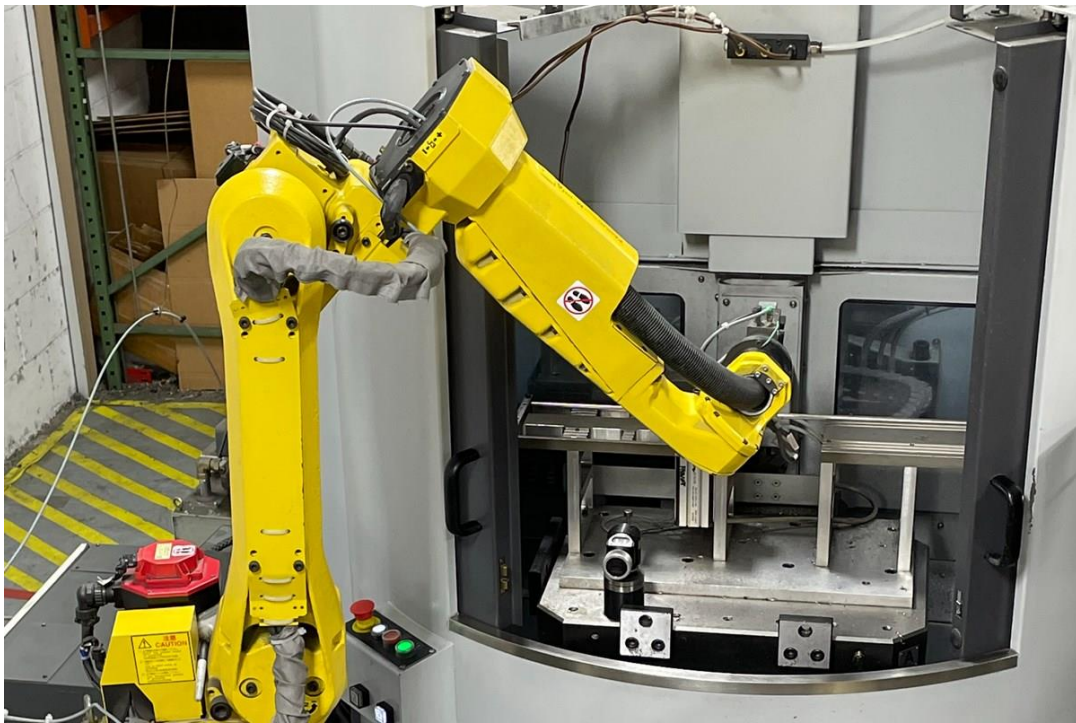
Figure 2: Robotic Arm with CNC Tool
