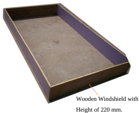
Fig. 3.A: Frame of Windshield
