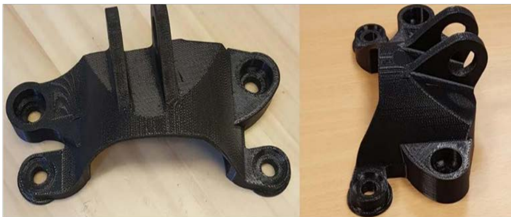
Figure 6. Engine Bracket after Fused Deposition Modelling (Additive Manufacturing) [16]
