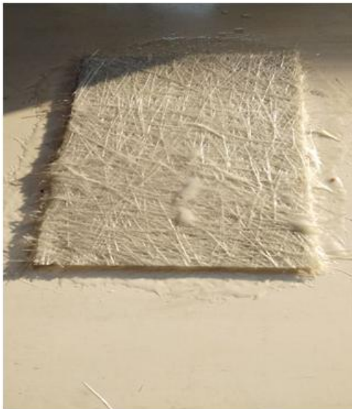
Fig.1 Sheet of chopped glass fiber
