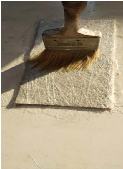
Fig 2. Application of epoxy on chopped Glass fiber sheet
