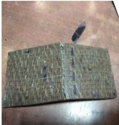
Fig. 9 Specimen after test from jute side
