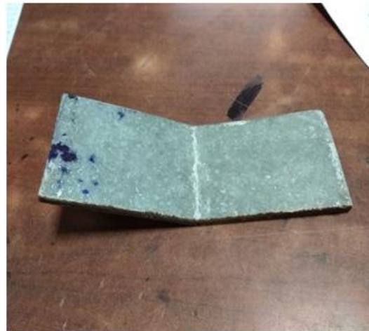
Fig.10 Specimen after test from glass fiber side
