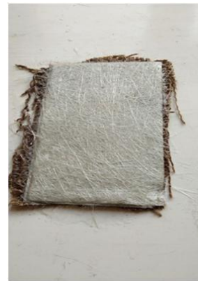
Fig. 3 Jute placed on glass fiber sheet
