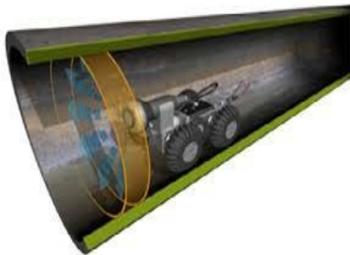
Figure 6. Autonomous/ Tele robotic concept design for AC duct cleaning
