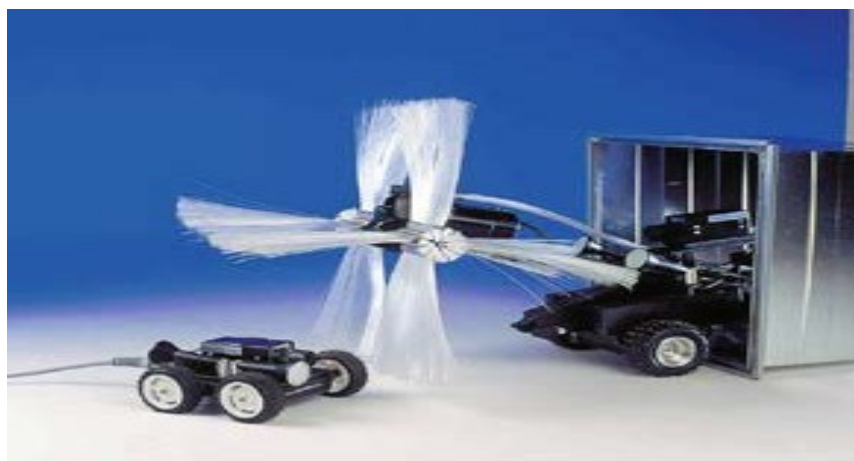
Figure 5. Small inspection robot and cleaning robot
