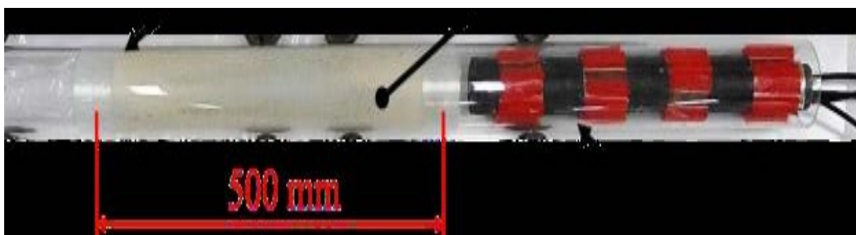
Figure 4. Experimental arrangement for duct cleaning
