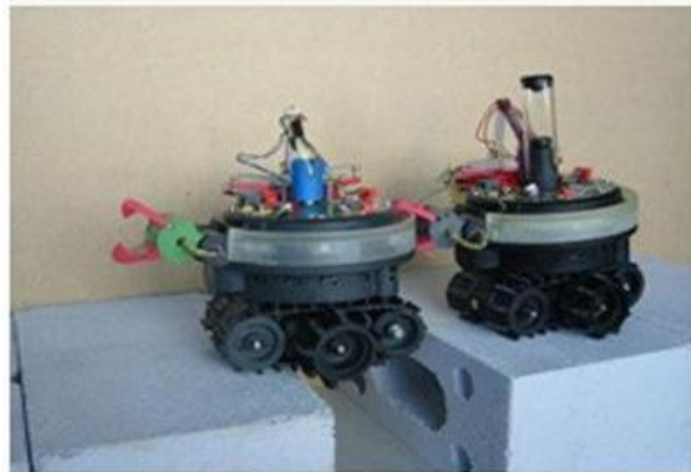
Figure 13. Swarm collaborate to pass an obstacle[14]
