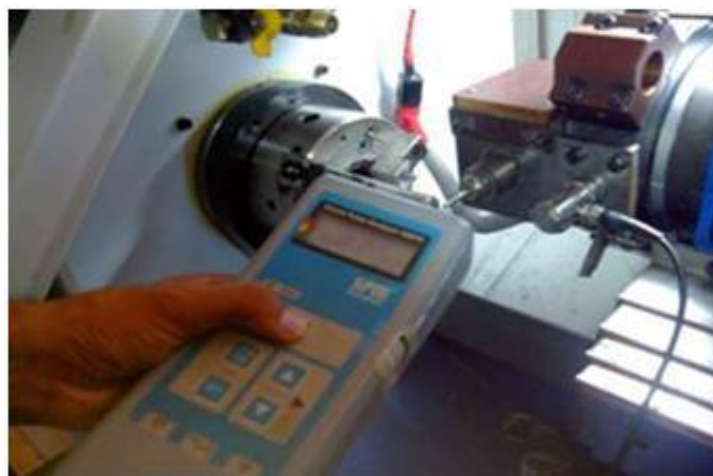
Figure 3. Vibration level recording using SPM
