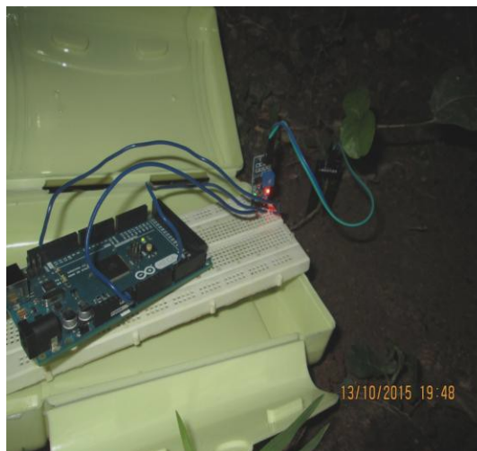
Fig. 10: Soil moisture sensor experimental setup: The probe is fixed in the soil and soil moisture is measured.
