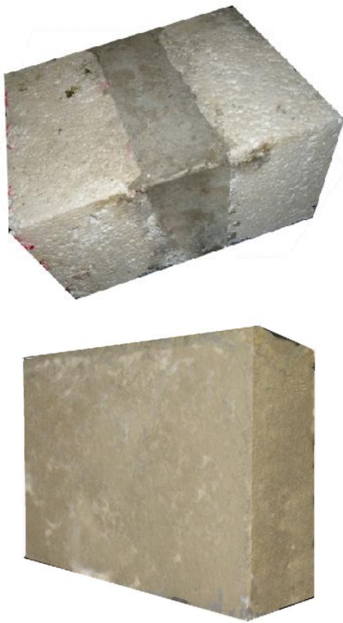
Figure 4b: Typical ICF model after casting and plain concrete
