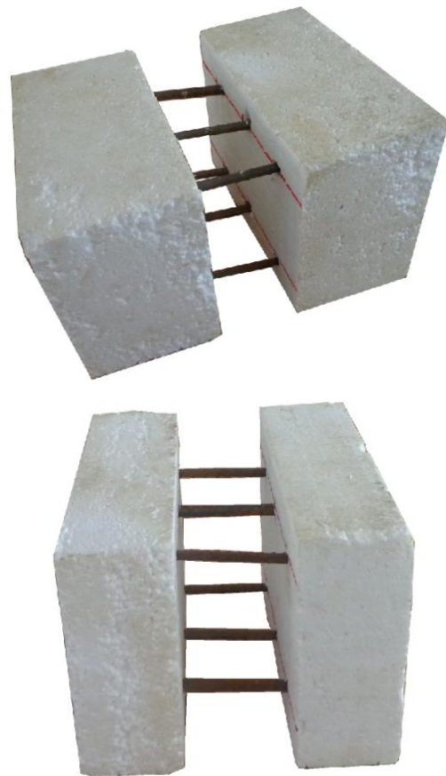
Figure 4a: Typical ICF model before Casting
