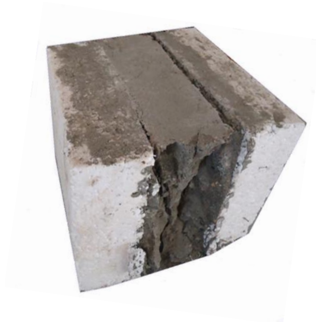
Figure 6b: Test Specimen using 60 mm EPS Sheet
