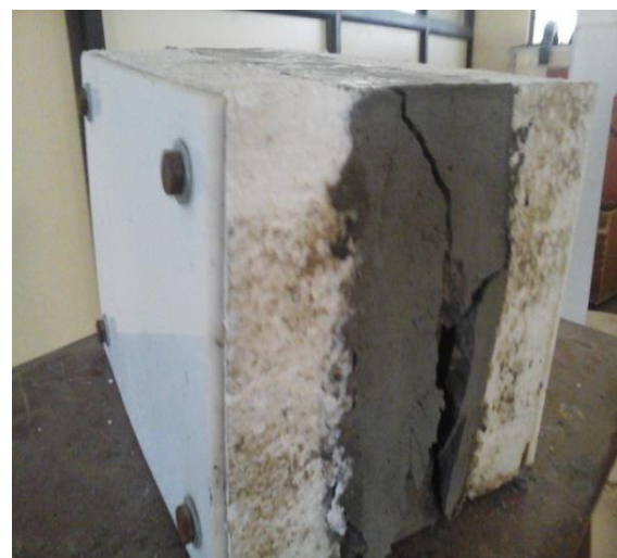
Fig 14: Side view of sample after sheet testing
