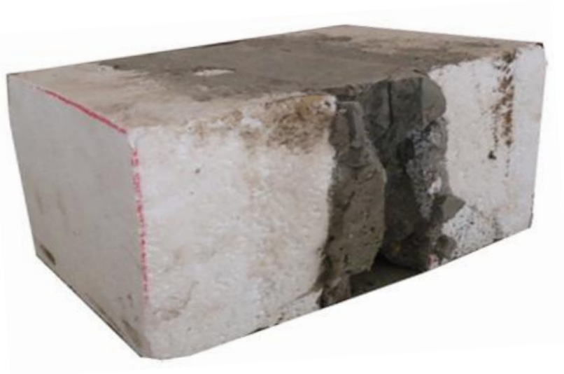
Figure 6a: Test Specimen using 100 mm EPS Sheet
