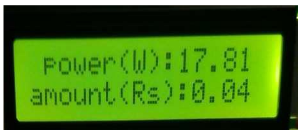
Fig. 5 Display of power consumed and the amount for the power consumed on LCD
