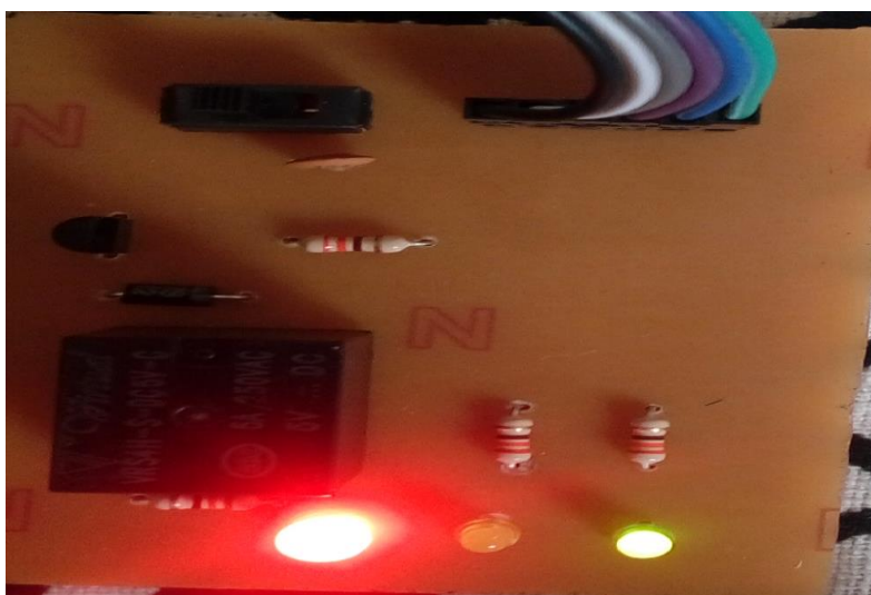
Figure 5: Red Light Indicates Ignition is ON and Yellow Light Indicates High beam
