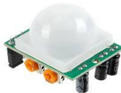
PIR (passive Infra Red)sensor :-
