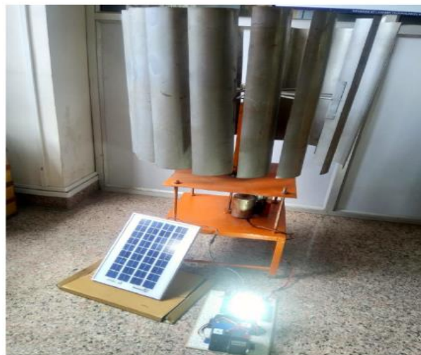
Fig 8: Whole set-up of VAWT and solar panel
