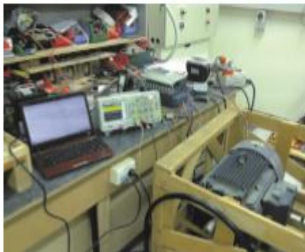
Figure 1: The industrial setup for induction motor experiment.
