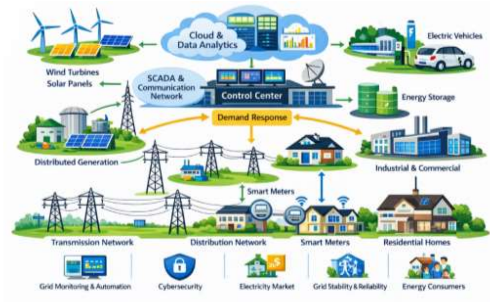
Figure 1: Smart Grid Architecture with Renewable Integration
