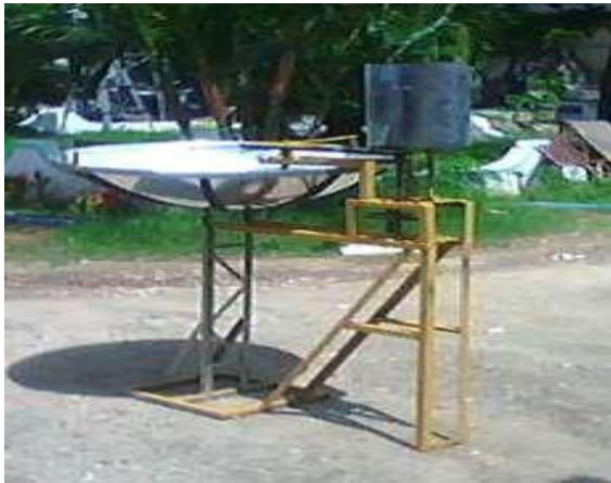
Fig.2. Experimental setup of the pyroelectric energy harvesting system
