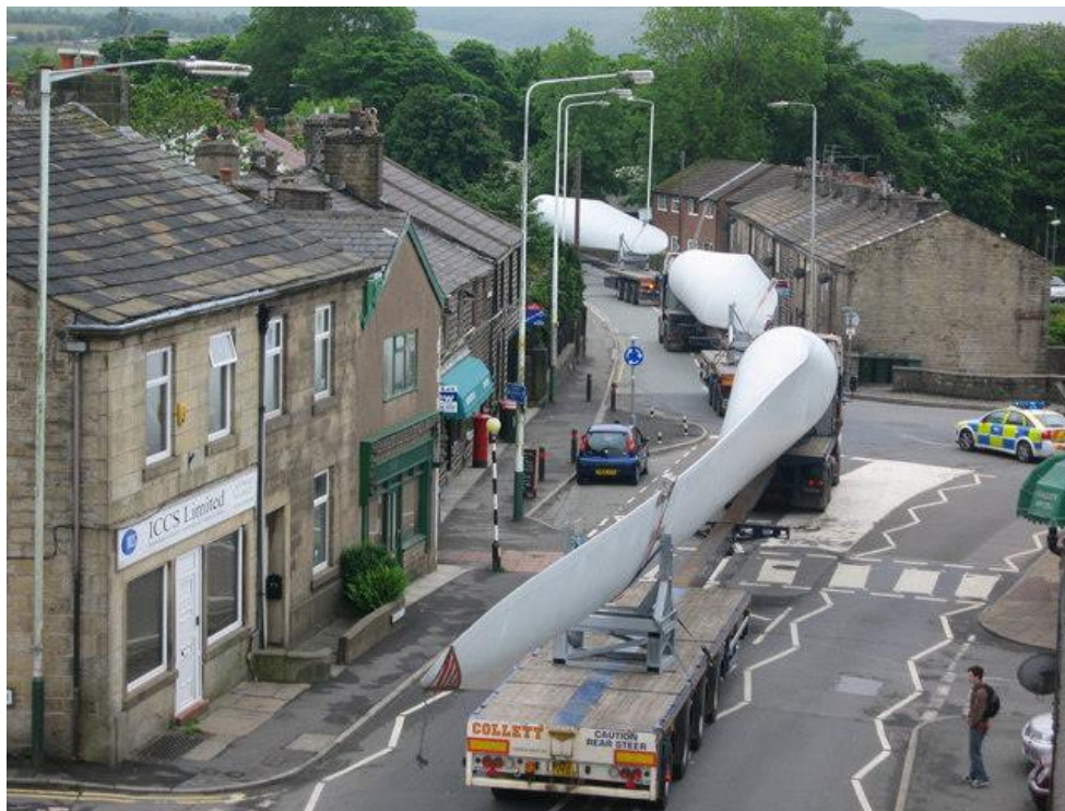
Fig. 5: Turbine blade convoy passing through Edenfield, England (Source: Wikimedia Commons)
