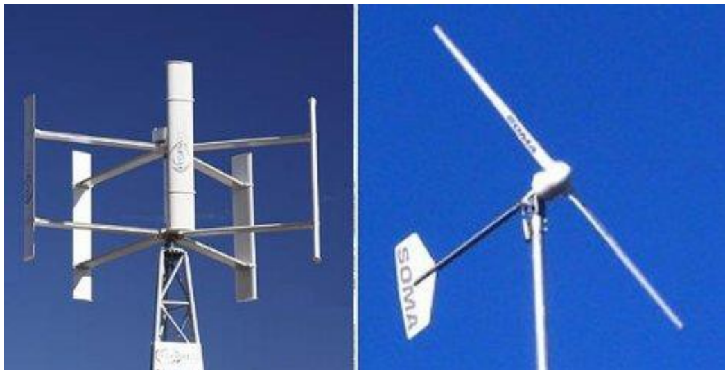
Fig 3: Vertical and horizontal axis turbines used for residential electricity generation
