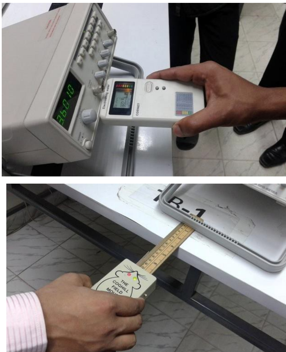
Figure 1: Electromog RF/LF Field Strength power meter Dual mode RF power meter & LF gauss meter ED-78S measuring magnetic field in front of Lab equipment (top image) and the COGHILL FIELD MOUSE measuring the EF and MF threshold values (see the red and green lights). Green light indicates that the EF threshold has reached while the MF threshold reading still showing red i.e. threshold not reached yet (bottom image).
