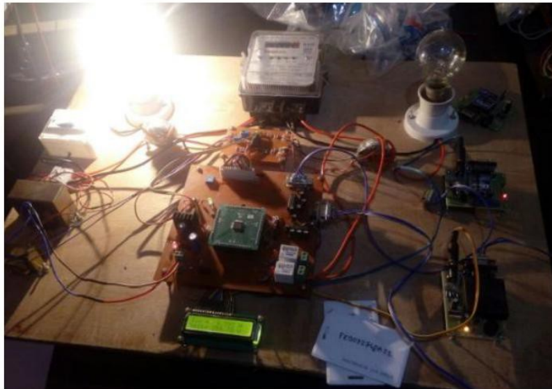
Fig. 9: Automatic Meter Reading when Load is ON
