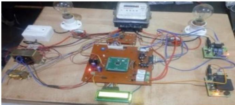
Fig. 7: System Hardware Transmitter and Receiver
