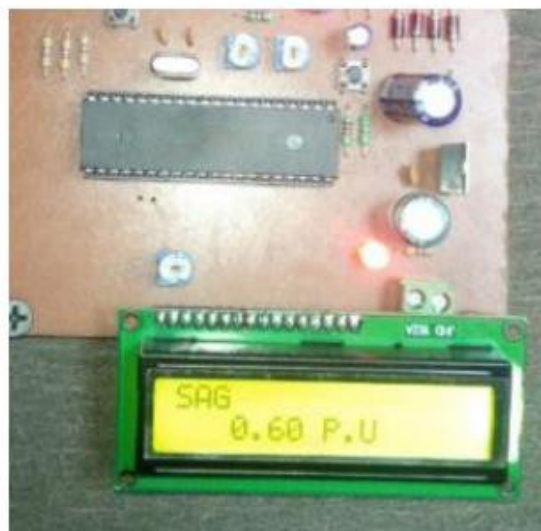
Figure 5 Hardware output for voltage sag.
