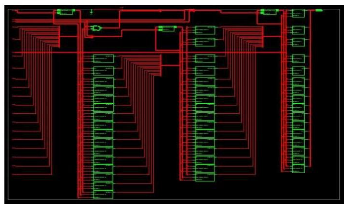
Fig.5 Internal RTL schematic of Shift-Add multiplier part 2
