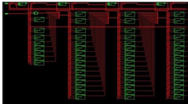
Fig.4 Internal RTL schematic of Shift-Add multiplier part 1
