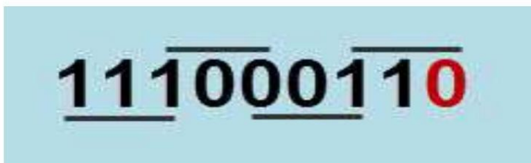
Fig.7 Bit pairing as per Booth recoding
