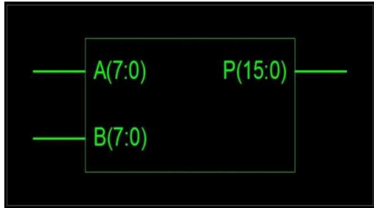
Fig.3 RTL schematic of Shift-Add multiplier
