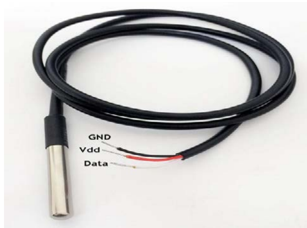
Fig -3: DS18B20 Temperature Sensor
