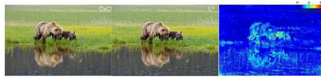
Fig. 4 Approximating DxO pipeline with L^3 local linear transforms
