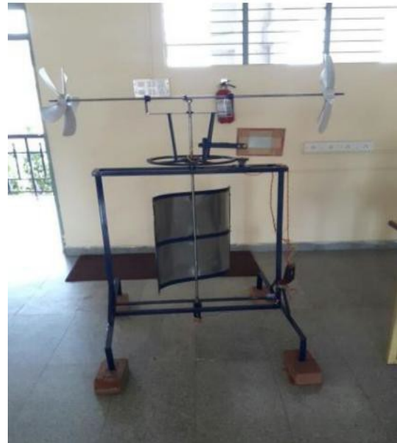
Fig-7: Multi Rotor Wind Mill Power Generation system
