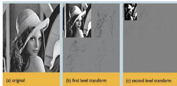
Fig. 6 Images with two levels of lifting
