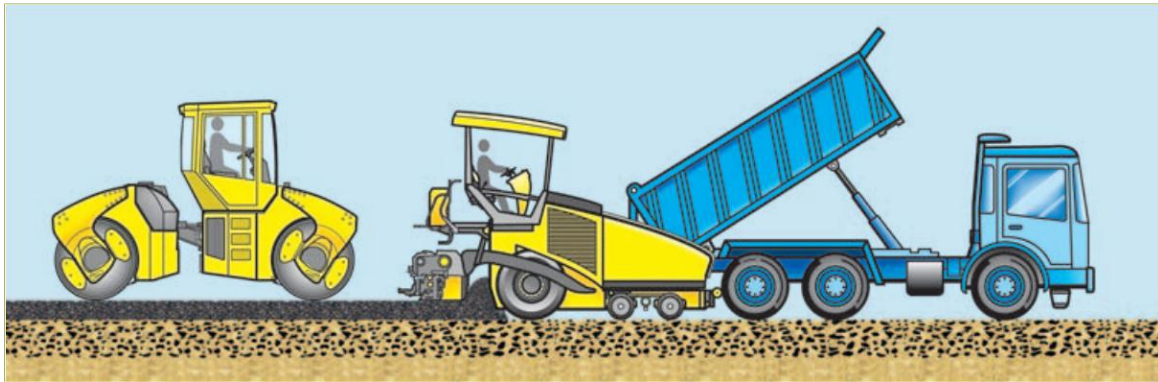
Fig 1 Working of paver and double drum
