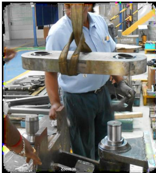
Fig 11 Nylon strap used to lift link rod at mule
