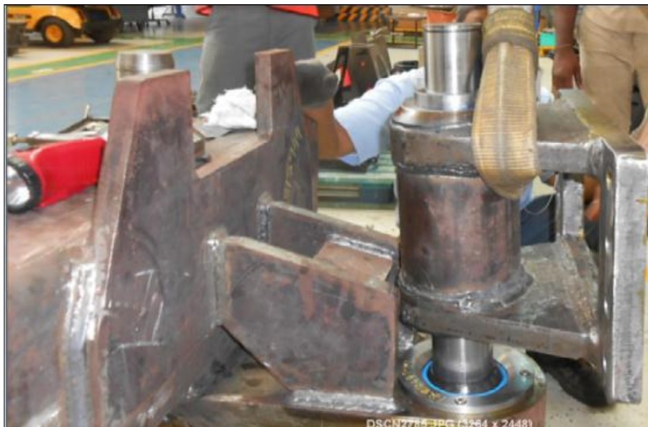
Fig 7 Lifting of modeled swivel casting along with articulation pin without fixture at mule
