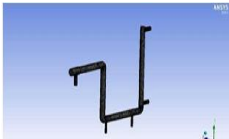
Figure 2 (b): Meshing of circular duct.
