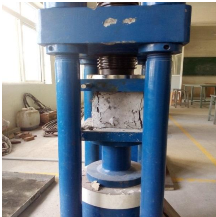
Fig1. Testing of concrete cube specimens in compression testing machine
